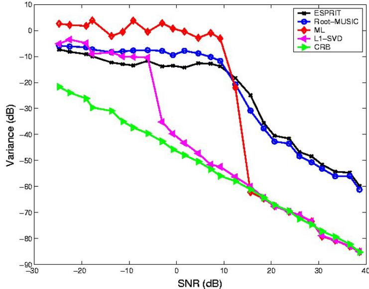
**Fig. 3.** Plots of variances of DOA estimates versus SNR, as well as the CRB, for two correlated sources. DOAs:  $42.83^\circ$  and  $73.33^\circ$ , variance for the source at  $42.83^\circ$  shown.
