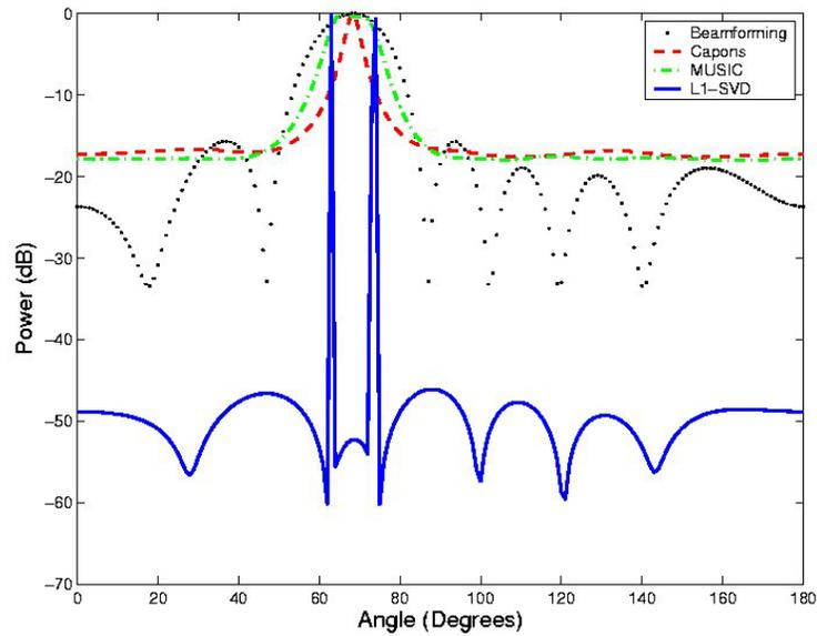
**Fig. 2.** Spectra for correlated sources, SNR = 20dB, DOAs:  $63^\circ$  and  $73^\circ$ .
